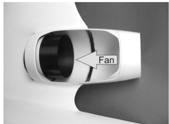
Cut out the nozzle (14) from the film supplied, and stick it to the mantle ring of the ducted fan unit from the rear using adhesive tape.
