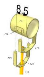
Glue one part 224 horizontally to housing 223 and drill through housing. Drill one hole through housing on opposite side, use hole to position second part 224, then glue in place.
