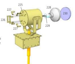
Glue back panel 225 to housing 223. Glue handles 226 and fasteners 227 in place as shown. Paint search light.
